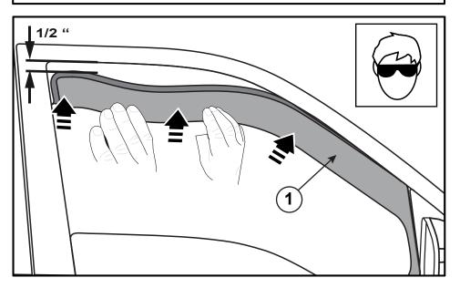
4. Start inserting the Visor (1) by carefully rotating it into the door glass seal.
