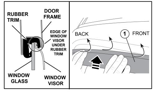
5. Ensure the Visor (1) is located in the outermost section of the door glass seal.
