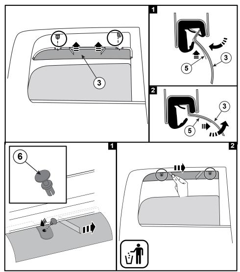
6. Pull the bottom outwards while raising and lowering the window a minimum of 5 times.
