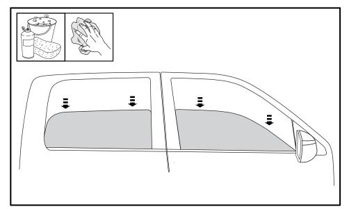
Fit the Visor (1) behind the mirror.Ensure the bottom edge locates on top of the lower window molding.
