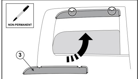
2. Pull the glass seal away from the door frame and install the clips into the seal at the noted locations.
